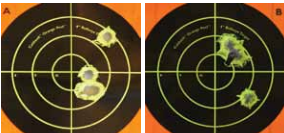
Left: 300gn Hornady- 4 shots into 15mm then a flyer. Right: 300gn Woodleigh-4 shots into 12mm and another pesky flyer!
