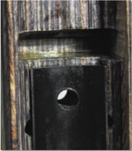
The recoil lug slots into this recess in the stock, which is epoxy-resined for additional strength.
