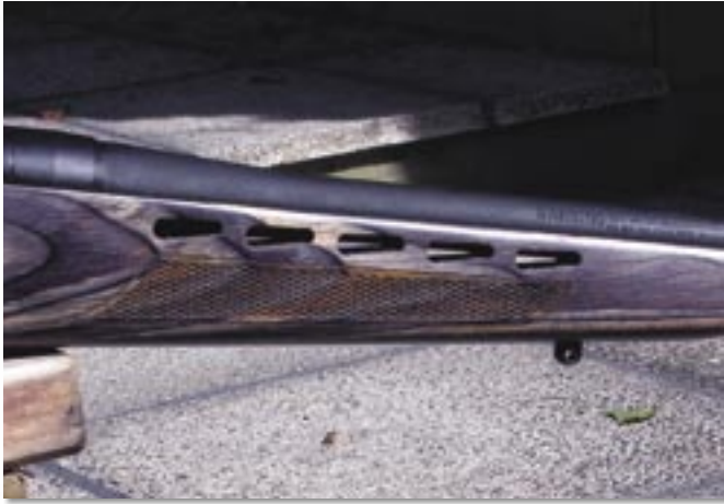
The forearm is free-floated, and ventilated to allow barrel heat to escape.
