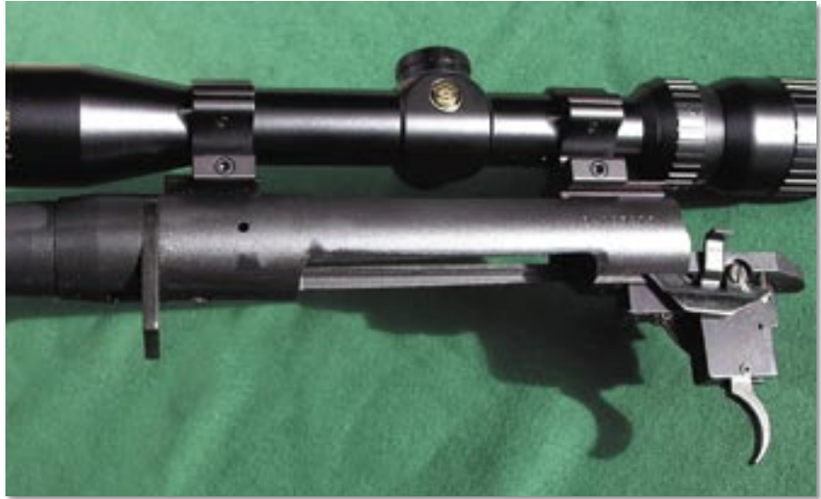
The tubular receiver is machined from bar steel and has a Remington style recoil lug.
