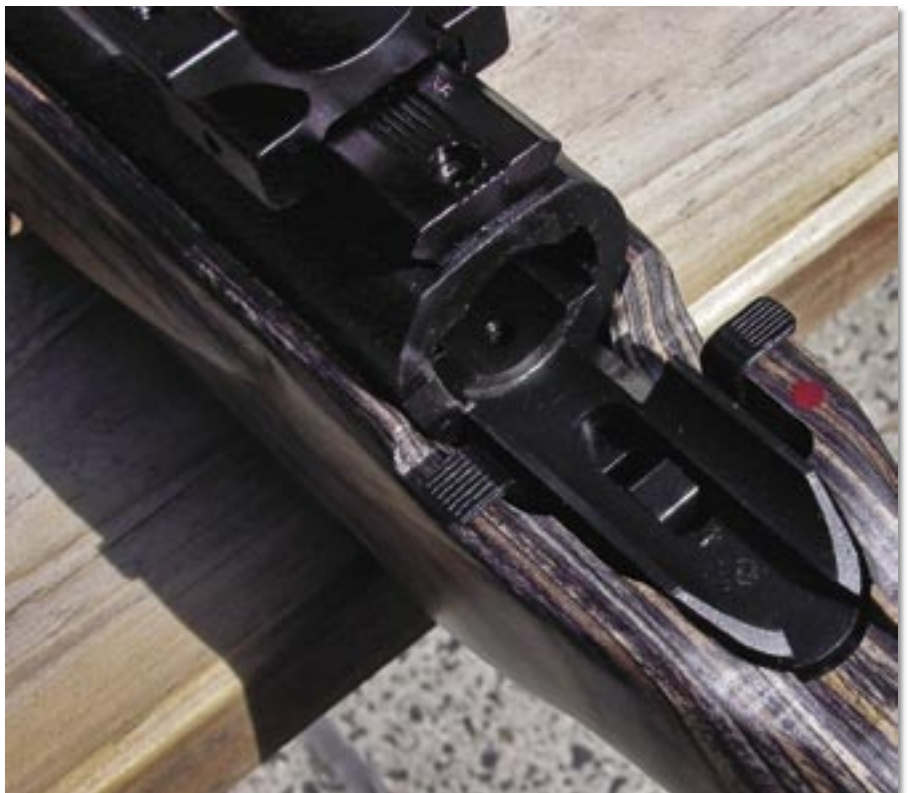
The bolt release lever is located on the left rear of the action, with the two-position safety catch on the right.
