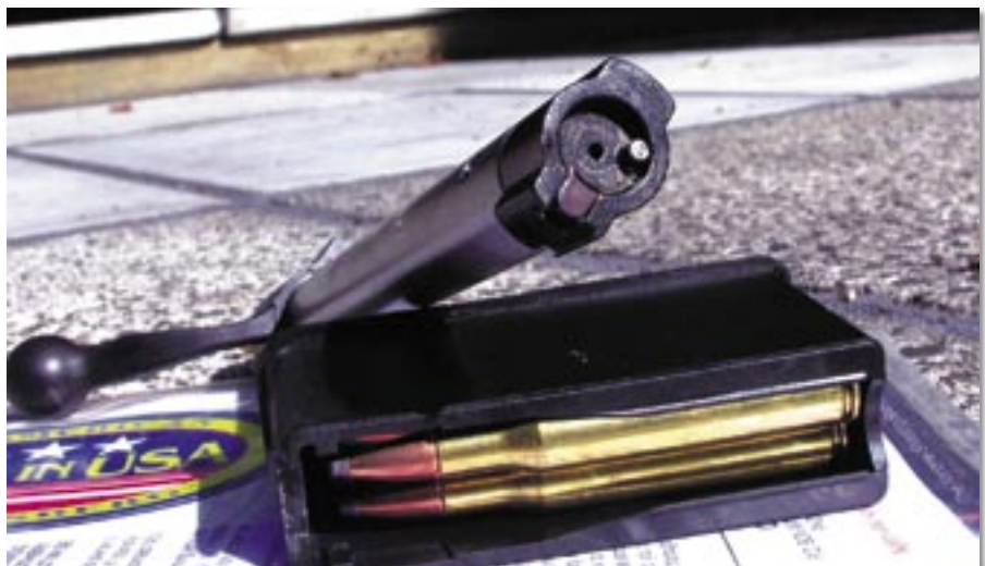
The bolt features an extractor housed in the right side lug, and a plunger-style ejector.
