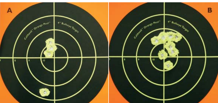
Left: 5 shots at 50 meters – first shot low from clean barrel. Right: 10 shots rapid at 50 meters.
